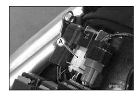
• Set the hand tester to the  $\times$  10  $\Omega$  or  $\times$  100  $\Omega$  range and connect it to the diode unit terminals to check the resistance in both directions.
