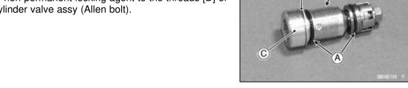
• Hold the cylinder unit [A] by using the fork cylinder holder [B], install and tighten the cylinder valve assy [C].
