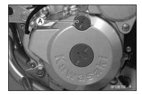
• Attach the timing light [A] to the ignition coil lead in the manner prescribed by the manufacturer.
