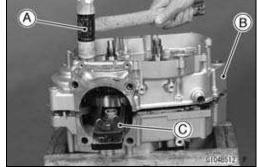
• Tighten the crankcase mounting bolts starting with the ones around the crankshaft, and then the farther ones.
