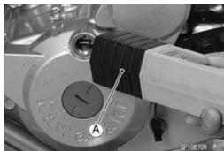
• Run the engine at the speeds specified and note the alignment of the ignition timing mark.
