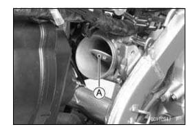
• When install the air cleaner duct, fit the air cleaner housing projection [A] to the air cleaner duct groove [B].
