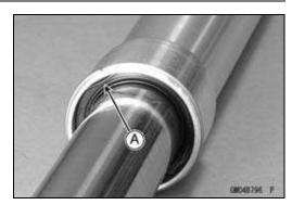
OHolding the inner tube [A] by hand, pull the outer tube [B] several times to pull out the outer tube.
