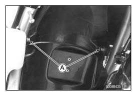
Remove: Bolts [A] Rear Fender Rear [B]
