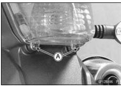
• Clear the stoppers [A] from the tail/brake light body with a screwdriver [B] to remove the lens [C].
